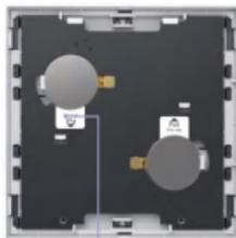
Remove the battery insulation sheets before use.
